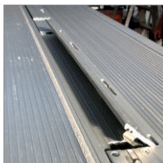
28 Automatic trolley stop 45° (2 stops).
