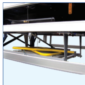
Structure to be fixed under the semi-trailer body to house 2 guards and the side ramp
