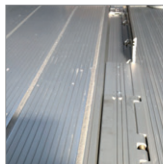
29 Automatic trolley stop 90° (2 stops).
