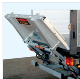
33 Folding cantilever platform for drop side body.
